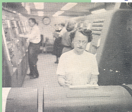
Violet Young, one of eight Services girls who operate wire room, checks copy at top-line printing machine. In the background are 12 tables and 24 reperforators receiving tapes.
